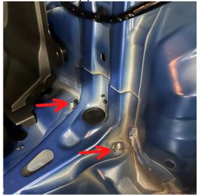
4. Push down on the control arm and remove shock from vehicle.
