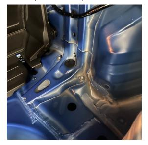
2. Remove the nut/bolt that attaches the shock(17mm) and sway bar endlink(14mm).
