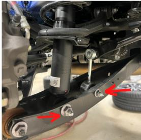
3. Remove two upper nuts that fasten top mounts to chassis. (14mm)
