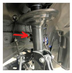
**4**. Remove two lower 19mm clevis nuts/bolts.
