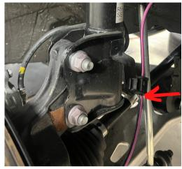
3. Remove the 17mm nut/bolt attaching the sway bar to the strut.
