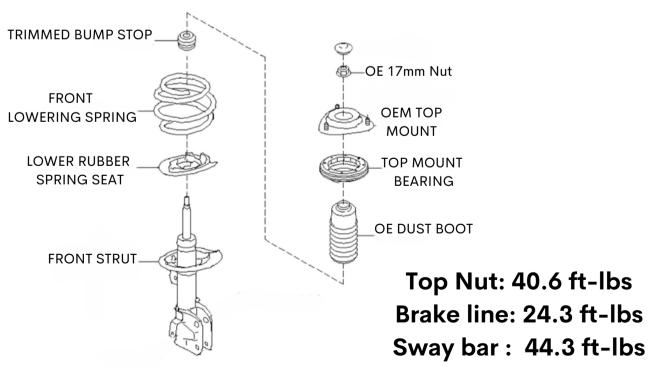
Top mount to chassis nuts: 23.6 ft-lbs Lower clevis bolts/nuts: 114.3 ft-lbs
