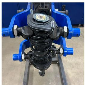
6. Remove top mount, spring, dust boot, and bump stop from shock.
