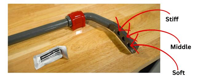
**5.** Re attached the OEM mounting brackets onto the new bushings and carefully guide the sway bar back into place. Secure the sway bar by re installing the (4) 12mm bolts on the mounting bracket to the chassis. **DO NOT FULLY TIGHTEN**
