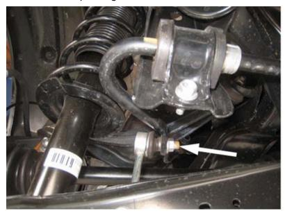
**3.** Remove (4) 12mm nuts that secure the sway bar mount to the chassis and carefully pull out the OEM sway bar along with the mounting brackets.
