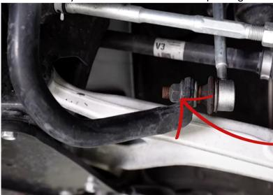
Remove 17mm nut on each side
