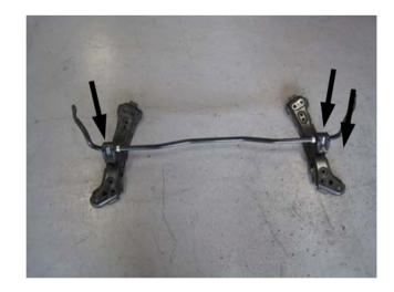
**6.** Remove the new RCE bushings and apply a generous about of the supplied lubricant on the inside of the bushings. Reinstall on the sway bar after proper lubrication.
