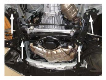
**5.** Remove the (2) 14mm bolts on the front and (2) 12mm nuts on the back side securing the sway bar on the sub frame.
