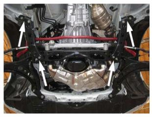
13. Bolt end links to the sway bar in the desired position and tighten. 34 ft-lbs
