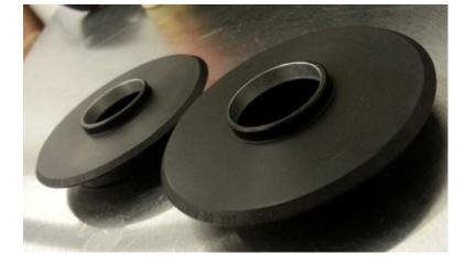
7. Place the adapter on top of the coilover spring so that it sits snugly inside the spring. Then place the Group-N top mount on top of the adapter so the small round protrusion sits inside the hole in the bottom of the mount. PLEASE NOTE: the rounded portion of the top mount should face outward, in line with the lower clevis tabs on the
