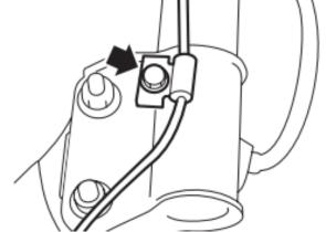
2. Remove the two 19mm nuts/bolts that attaches the front strut to the hub
