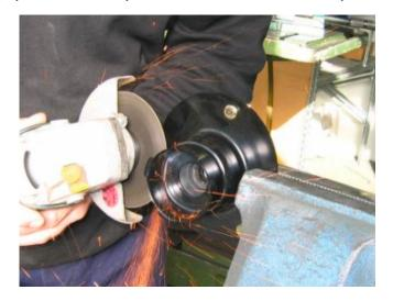
4. After the cut is complete, use a sanding disc to smooth out and flatten the cut. Be sure to remove any peaks or sharp edges:
