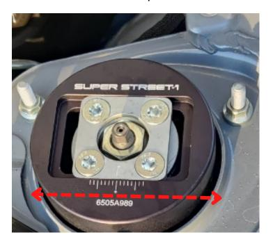
**Torque Spec**Torx Bolt: 17 ft-lbs
