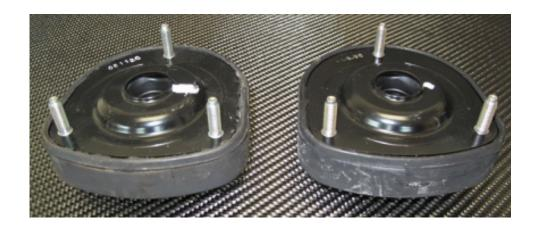
1. Begin the modification by removing the outer rubber isolation cover. You can simply grab it around the edge and pull it firmly downward. You will be left with the
