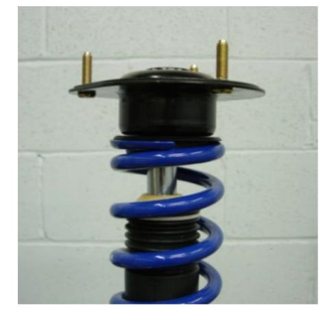
8. Thread top nut onto strut shaft. Use strap wrench to prevent spinning and tighten. **Torque spec is 26 ft-lbs**
