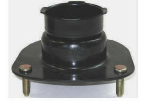
2. The mount is separated into two individual steel stampings, with the bottom portion shaped like an inverted cup. You will be cutting the mount where the two stampings are joined, marked with a dotted line shown:
