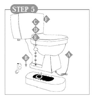
STEP 5: Re-install the Toilet onto the Spacer
