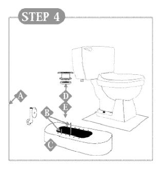
STEP 4: Install the Spacer and Soil Pipe Extension
