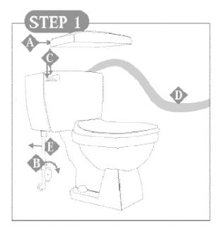
STEP 1: Disconnect Water Line from Toilet and Empty Toilet of Water
