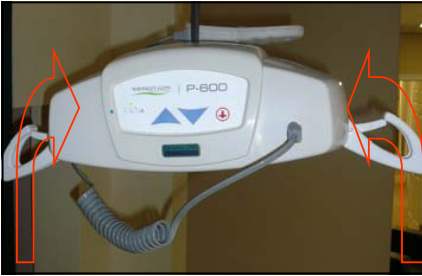
Figure 16A - P-600 with hooks in normal position
