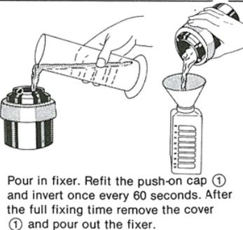
Pour in fixer. Refit the push-on cap (1) and invert once every 60 seconds. After the full fixing time remove the cover (1) and pour out the fixer.
