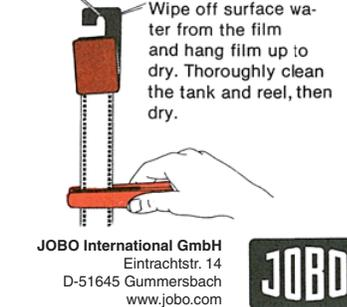
Wipe off surface water from the film and hang film up to dry. Thoroughly clean the tank and reel, then dry.
