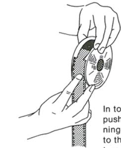
In total darkness push the beginning of the film into the first groove turn.
