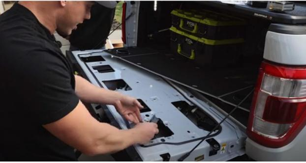
Note: for added sealing capabilities, pickup these sealing washers and place them under each bolt head, when reinstalling the tailgate panel. <a href="https://www.mcmaster.com/94733A719/">https://www.mcmaster.com/94733A719/</a>
