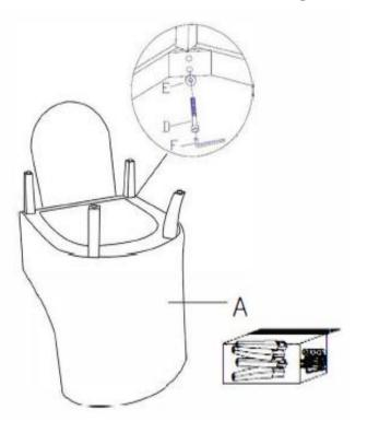
Step 3 Check all the bolts are tighten securely in position, put the dust cover back to the position. Upright the chair and make sure the chair is stable.
