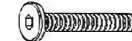
6 x3 Allen bolt M6*40mm * x3 Vis à tête creuse hexagonale M6*40mm x3 Perno Allen M6*40mm
