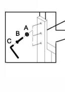
NOTE: Must tighten screws periodically with use. Screws will become loose, check tightness of all Page: 1 of 2 screws every 6-8 weeks.
