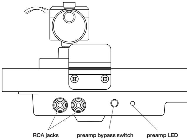
The built-in preamp is set to “on” out of the box. To disable it, press the bypass switch. The preamp is enabled when the LED light is on.
