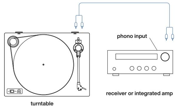
You can also connect your Orbit directly to any receiver or amplifier that has a clearly marked “phono” input on the back.
