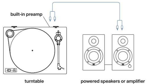
With the built-in preamp enabled, you can connect your Orbit directly to powered speakers or an amplifier using the included RCA cables.
