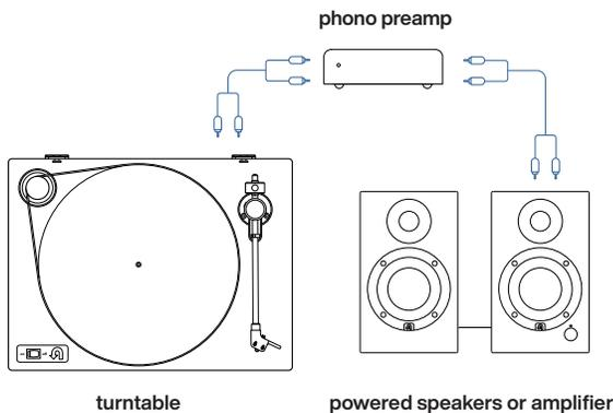
If your Orbit doesn't have a built-in preamp, you can connect it to a standalone phono preamp then connect to powered speakers or an amplifier.
