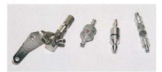
Step 10: I use a fuel filters for a clean oil flow, a check valve to prevent muffler pressure from pushing oil back into the pump tubing, and most importantly, a remote needle valve assembly to regulate the oil flow. If you don't meter the flow properly, the oil can cool off the muffler and reduce the amount of smoke it generates. This is much better than using a clamp on the oil tubing. I used a needle-valve assembly from an old O.S. .61 engine. It works great!
