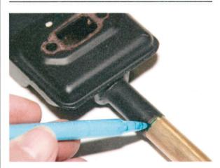
Step 6: To provide a baffle tube, a large brass tube is slipped in to fit into the muffler and the fit should be snug. The tube is longer than the internal tube already in the muffler. Slip it into place, bottom it out and then mark the length. Use a K&S Tubing cutter and cut it to length.
