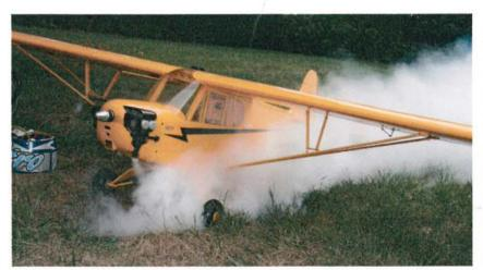
Step 13: Check out the smoke density! This is what it looks like with the oil flow almost completely shut down (only one turn open). This setting gives a lot of "smoke-on time" and the 10-ounce tank lasts more than 10 minutes. The system works great and when you switch the smoke off, it takes about 5 to 7 seconds for the smoke to stop completely.
