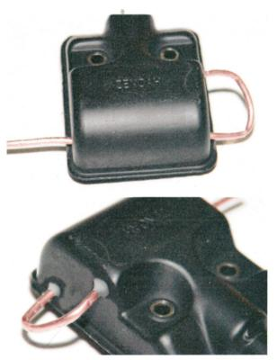
Step 5: Here you see the injection tube installed and ready to be sealed with JB Weld metal epoxy. Be sure to clean the injection tube as well as the surface of the muffler. Build up fillets around the tubes/holes areas. Smooth the fillets with a wet finger and then set aside for 24 hours to fully cure.
