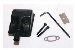
Step 1: Here's the stock muffler removed from the engine and cleaned up with some MEK solvent to really degrease it. I used a new single-edged razor blade to remove the old exhaust gasket. Here you can see the new one I will add after the muffler has been modified.
