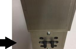
Fuel Barbs: Connect fuel lines to fuel container and to the model fuel tank. Make sure pump is off prior to connecting or removing fuel lines.
