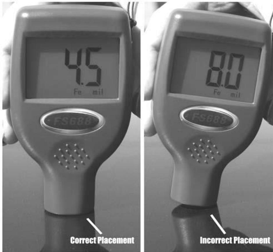
As I attend auctions I can't believe the number of dealers I see using a gauge incorrectly. If you are looking at a vehicle and you see a reading that appears to be high, I suggest lifting the gauge a few inches and then pressing it on the surface again; making sure that it is flush.
