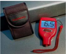
To be successful with a Paint Meter you must learn to look for large changes in the readings. Paint thickness usually varies about 1 mil to 1.5 mils on most cars. When a panel has been refinished you will usually see a jump of 2 mils or more.
