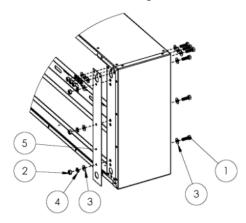
Attach the vent hood dire tly into the spacer through the mounting holes located on the rear hood cover plate. Fasten and tighten all hex nuts. Reference the parts list below to identify the hardware included with your wall mount spacer.
