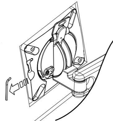
**6B** Adjust VESA friction to suit the offset weight of the monitor
