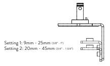
INSTALL CLAMP SCREW AND CLAMP
