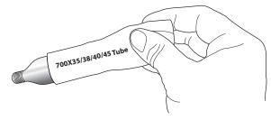
Prevent Rattling. Place supplied recycled Tube over CO2 Canister and Slimline Multitool
