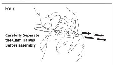
To fix the Aeroclam to your saddle you must separate the Aeroclam halves. Hold the top section in your left hand and slide the bottom section directly away from you with your right hand.
