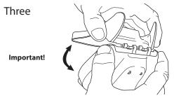
**Important!** Do not open the Aeroclam halves any more than shown above as separating the top and bottom sections will become difficult.
