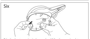
Take the clam top section in the same hand & line the mounting slot up with the nut in the clamp then loosely tighten the bolt [must use washer!].
