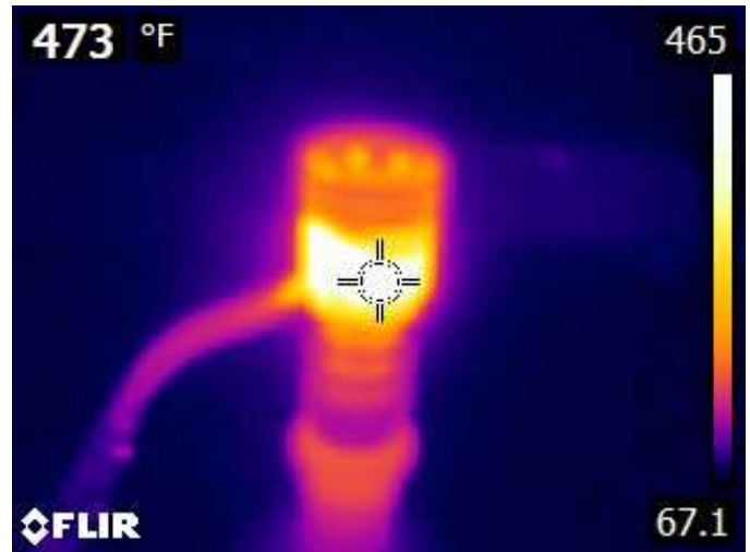
Fig 2a. An Infrared thermal image of Auber 15.8 mm coil/nail assembly. SV =550F. The temperature reading at the top left corner is from circle at the center.
