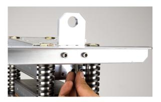
Use Allen Wrench to tighten in place, then hold the second bracket in place with the handle installed.
