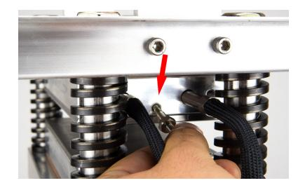
On each side of each plate there are recessed screws which will tighten onto the heating rod from the inside and keep them in place. Check that you have done it correctly by lightly pulling on the heater rods. If they do not come out of the plate, you are set.
