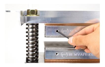
This is what it should look like with the heating rods and thermocoupler installed correctly.
