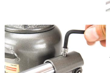
Tighten the Pump Handle in place.
