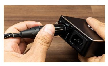
1. With all switches off, plug in your coil to the back of the controller.
