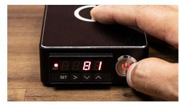
3. Once Power button is turned on, it will display the ambient temperature of the coil.
