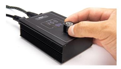
5. Use rotary knob to dial-in target temperature.
