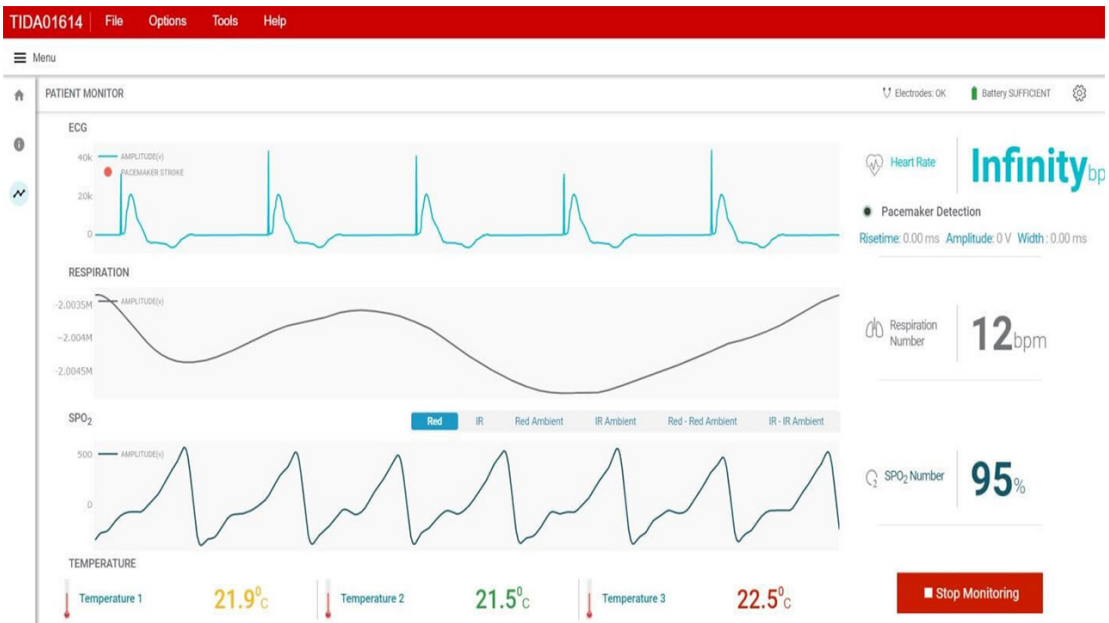
Figure 3: GUI displaying ECG, PPG, pacemaker, heart rate and skin temperature
