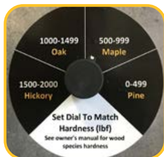
Easy adjustment dial for cycle speed for different wood species
