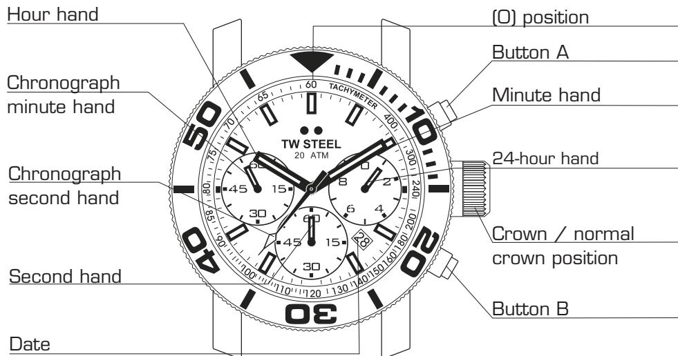
chronograph second hands can be advanced rapidly by continuously pressing button A or B. Once the hands have returned to the (0) position, return the crown to its normal position and screw the crown cap clockwise back to the case.
