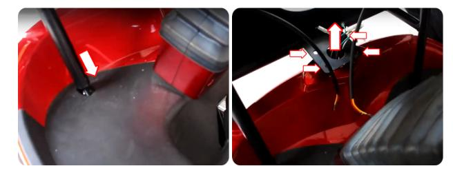
Locate the threaded ends of the support arms now located on the under side of the body, stack and add 2 nuts per thread and tighten.
