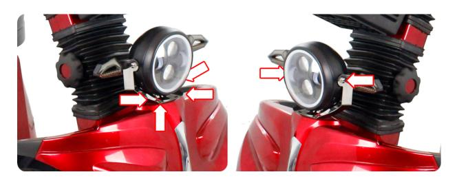
Headlight - 1 Large White connector & 3 individual pin connections Turn light - 2 individual pin connections each (please note which set is for which side for correct signal operation)
