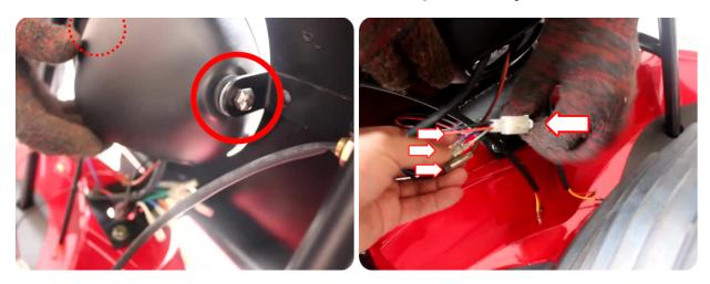
Reconnect the large white connectors and 3 corresponding pin connections as noted earlier. Reconnect the correct turn signal to each set of signal connections and carefully tuck wires back below the body. Insert and secure the reflectors into the holes front plate.
