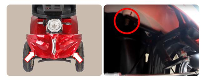
To reinstall the headlight, first insert a washer in between the headlight and mounting bracket on the front plate cutout, aligning the holes in each. Then secure with the bolts previously removed.
