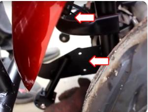
Locate the middle rear support arms. Tilt the seat forward, remove the installed rubber spacers and reinstall with one end of the support bracket underneath the spacer. Secure the other end of each support bracket to the rear roof support with a small bolt and nut.
