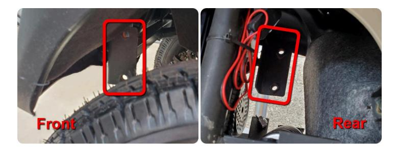
With assistance align the bumper below the mounting plates and line up the holes on the bumper with the holes on the mounting plate. Bolt upward into the nut welded into the mounting plate, 2 bolts per side, 4 per bumper.
