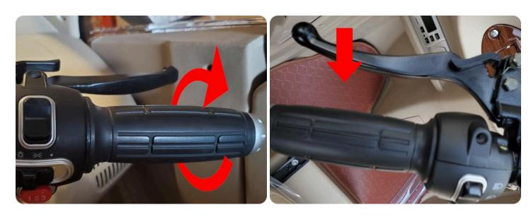
$\triangle$  Drive with care on slippery surfaces as it will increase the distance needed to stop, allow extra room for braking. When driving downhill, release the throttle & apply brakes to control the scooter's speed.  $\triangle$
