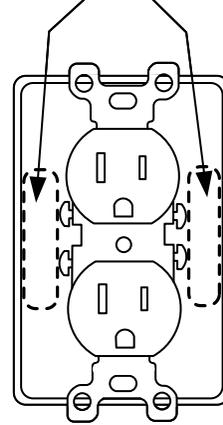
**STEP 3:** Remove existing coverplate from the outlet.
