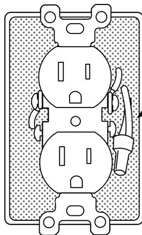
These wires may prevent the Product prong from contacting the screw terminal
