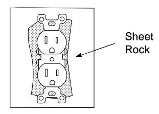
Obstruction 1: Sheet Rock or other wall coverings can prevent the prongs from passing around the outlet. This can be solved by removing the excess sheet rock near the screw terminals. If you are unsure of how to properly do this, please consult an electrician.
