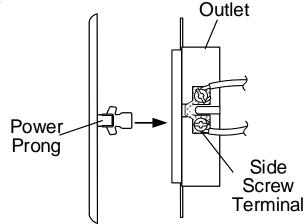
The power prongs slide around the side screw terminals and contact the lower screw heads to extract power for the Product.
