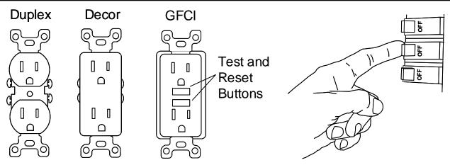
STEP 1: Select an outlet for the Guidelight will be installed over. The Guidelight is only compatible with standard duplex, décor, or GFCI outlets with side screw terminals.
