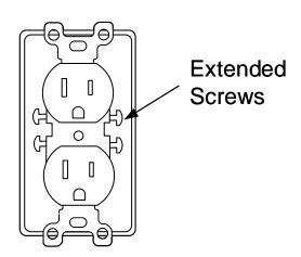
Obstruction 2: Screws may be all the way out and catch the ends of the prongs. To solve this, simply maneuver the prongs around the screws during installation.
