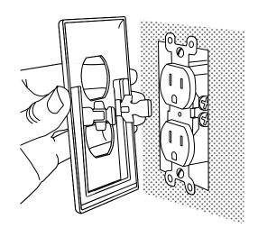
STEP 5: If clear, place the Guidelight over the outlet and secure with screw(s). Be sure that the prongs slide *inside* the electrical box.
