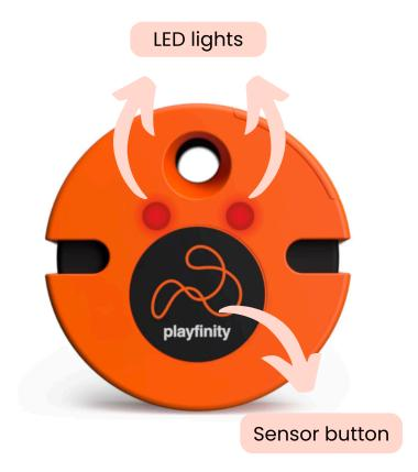
2. Now, remove the battery from the sensor. While pressing the sensor button, insert the battery again, and release the button once it is in its place, as shown in this video.
