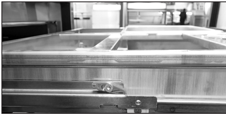
Fig. 1. Drawer retainer location. Retainer is engaged.
