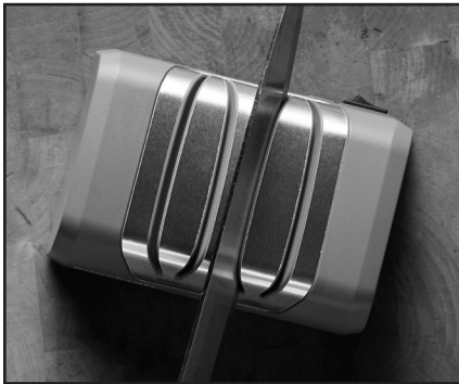
Figure 4. Knife in Stage 2. Use alternating sharpening strokes with modest downward pressure. See text.
