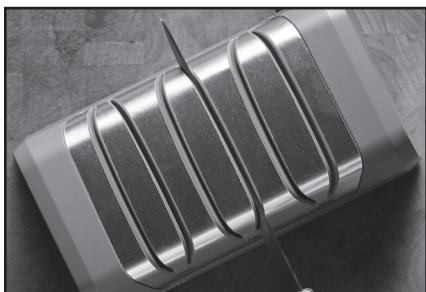
Figure 5. Inserting the knife in right slot of Stage 2. Alternate individual pulls in left and right slots.
