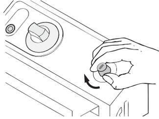
5. If unable to reset the temperature safety switch or if the switch continues to trip, contact Vollrath Technical Service.
