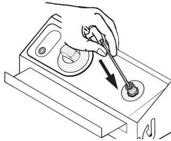
4. Replace the switch cover and secure by screwing clockwise.
