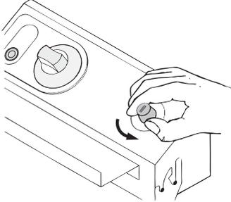
3. Use a pen or similar narrow tool to press the reset button down. The button should stay in the down (set) position.
