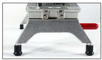
These slicers have four screws on each end that hold the blade assembly to the frame. To tension the blades, tighten the screws on the short leg end.
