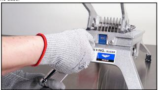
Remove the screws, washer plates, and o-rings from the short leg side.
