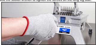
2. Tighten the screws until the assembly is tight against the frame.
