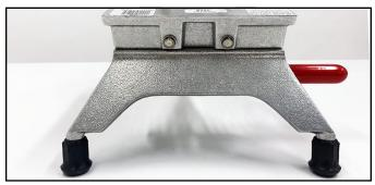
These slicers have two screws on each end that hold the blade assembly to the frame. To tension the blades, tighten the screws on the short leg end.
