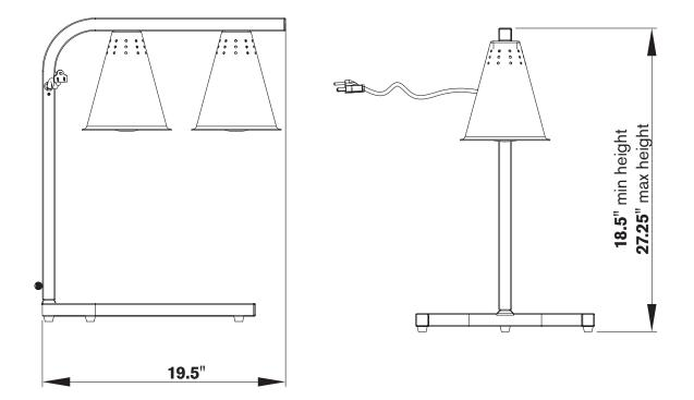
**Electric**: Attached 6-foot flexible, three-wire cord with ground plug (NEMA 5-15). **Construction**: Stainless Steel **On/Off Switch**: Easy-to-use and access
