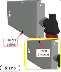
• Remove the snap-in fastener from the faucet side car and place into the hole directly above as shown.
