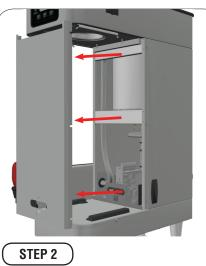
• Carefully remove the front panel of the brewer.
