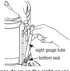
Press down on the sight gauge top to release the sight gauge tube. Remove the sight gauge tube and bottom seal.
