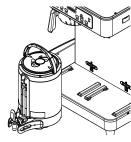
Place an empty server under the funnel. Rotate handle forward to lock the lid.
