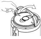
Completely drain the server. Rotate handle back to release the lid lock.
