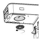
Once a week: Remove the sprayhead by turning in a counter-clockwise direction.
