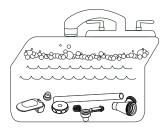
Transfer the sight gauge and faucet parts to a sink with a soap solution using a mild, non-citrus, non-abrasive, liquid detergent.
