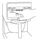
For two hopper grinders, select coffee type by pressing "RIGHT" or "LEFT" hopper.
