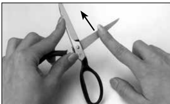
Figure 5. Carefully feel for a burr along the entire back of the blade. Note arrow for direction of finger movement when in contact with blade.
