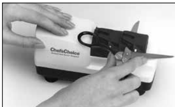
Figure 8. Start with the "Fine" Honing Stage.
