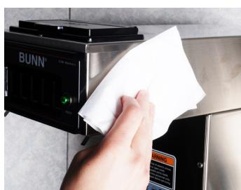
7. Use a clean damp cloth rinsed in mild, non-abrasive detergent to clean all outer surfaces.
