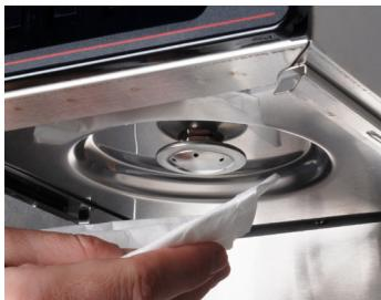
2. Use a clean damp cloth rinsed in mild, non-abrasive detergent to clean the sprayhead panel.
