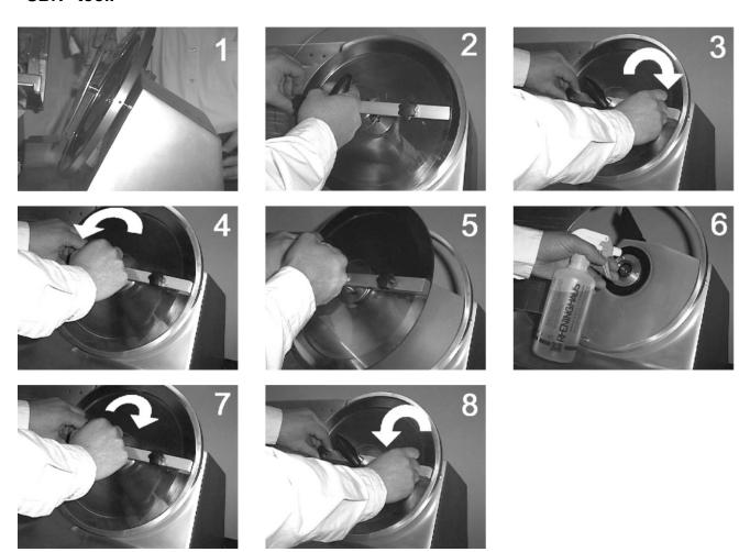
Lift the sharpener unit up off the blade.
