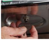
Use the blunt end of sprayhead cleaning tool to clean the sprayhead outlet fitting.
