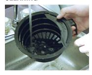
Clean and sanitize the funnel. NOTE: Do NOT clean this equipment with a water jet device.
