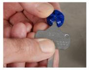
Use the pointed end of sprayhead cleaning tool to remove any mineral deposits from the sprayhead openings. The sprayhead openings must always remain open.
