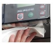
Use a clean damp cloth rinsed 3. in mild, non-abrasive detergent to clean the sprayhead panel.
