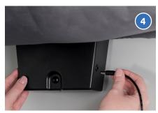
the safety button may not be completely set to allow PureAC to function properly. To resolve this issue, please make sure when installing the module that you push the module all the way back to approximately 1" from the wall and centered on the bottom of your wall mounted mini split system so that it attaches itself on the metal mounting plate.
