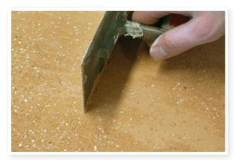
**1% Vermiculite** in Lime Wall Finish -fine-, tinted beige, scratching with the trowel in a 90° angle
