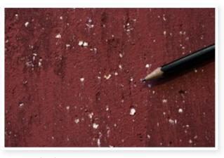
1% Vermiculite in Lime Wall Finish -fine-, tinted red
