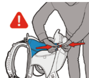
1.4 ⚠ Once the sidearms are resting in the cuffs, connect the red male buckle of the sidearms to the red female buckle of the cuffs. Your child carrier cockpit is now locked into the child carrying position.
