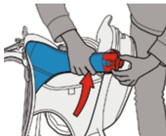
1.3 Rotate the sidearms up and insert the red end of each sidearm into the red cuff located on both sides of the child's head rest.
