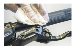
**13.** Check again whether the pressure point is now tight and defined. Then remove bleed block and insert brake pads. Then insert the wheel and turn the brake lever back to the desired position. Check the function again.
