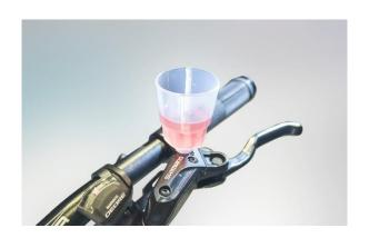
**11. After 2-3 times pulling** "pumping" on the brake lever, you should again have an optimal pressure point. Then you can close the funnel with the funnel stopper and carefully unscrew the funnel.
