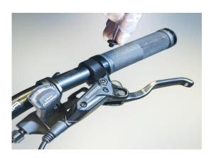
Now unscrew the funnel (do not insert the funnel plug into the funnel). It is sufficient to tighten it slightly by hand. Then fill the funnel approx. 1 cm high with mineral oil from the dosing bottle.
