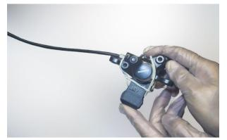
**Important for an optimum result:** Check again that the pistons are in the **end position**. If the pistons cannot be brought into the end position, the system on the expansion tank must first be opened. (See step 7)
