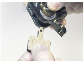
To avoid damage, never use metallic/sharp objects such as a knife or screwdriver.
