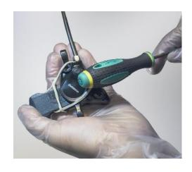
**Tip:** For an optimum bleeding result, pull the brake lever in between and release it again quickly to release air bubbles in the lever. Also carefully tap the brake line and the brake calliper, e.g. with the rubberised back of a screwdriver.
