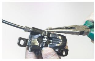
**3.** The pistons in the brake calliper must now be **pushed back completely**. Use the **bleed block** (6) or a piece of wood provided for this purpose.
