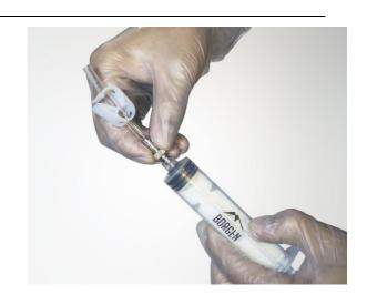
Now unscrew the cap completely from the bottle with the mineral oil (10) and fill the syringe with approx. 25 ml mineral oil. Close the clamp and make sure that there is no air in the syringe.
