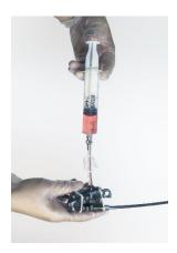
**Tip:** If foreign bodies such as metal chips or dirt particles are visible in the oil or the colour is not pink/red, seal the funnel with funnel plug and unscrew it. Dispose of old mineral oil properly and clean the funnel. Screw the funnel back on, remove the funnel plug and pour fresh mineral oil into the funnel.
