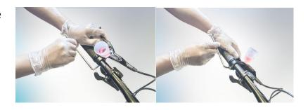
10. Close the vent screw as soon as no more air bubbles rise in the funnel or syringe. To do this, close the breather screw on the brake calliper. (Attention: Observe correct tightening torque - guide value: 4-6 Nm)
