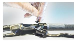
**Tip:** To avoid overtightening the screw without a torque wrench, clamp the hexagon socket only with 2 fingers (thumb and index finger) and tighten the screw very carefully.
