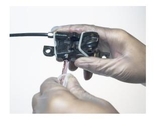
To prevent the hose from slipping off the nipple again during the bleeding process, attach the syringe to the frame or fork with the Velcro tape (8) included in the scope of delivery. The tip piston for pulling must point upwards.
