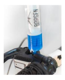
9-A Slowly pull out the piston of the syringe at the brake calliper. The oil now flows from the syringe body at the brake lever back into the syringe at the brake calliper. Now "pump" the oil several times from the bleeding syringe into the syringe body at the brake lever and back again (repeat procedure several times).
