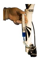
**8-A** Open the clamp on the tube and **slowly press the piston on the bleed syringe on the brake calliper**. The syringe body on the brake handle will now fill with mineral oil. You can now see that **small air bubbles** rising inside the syringe body at the brake handle.
