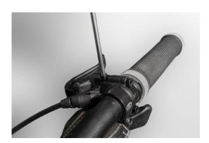
Now insert the syringe without the piston and without the M6 socket adapter (3) into the opening. Because of the conical shape of the syringe it can easily put on the EBT opening while still being firm and airtight.
