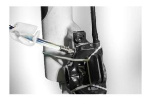
To make sure that the tube won't slip during the venting process, secure the syringes with the included Velcro at the bike frame. The syringe piston for pulling must face up.
