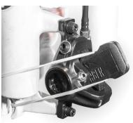
IMPORTANT FOR AN OPTIMAL RESULT: Check again whether the Pistons are in the right end position. If the pistons cannot be put in the right end position the system must be opened on the reservoir / EBT screw. (See step 7)
